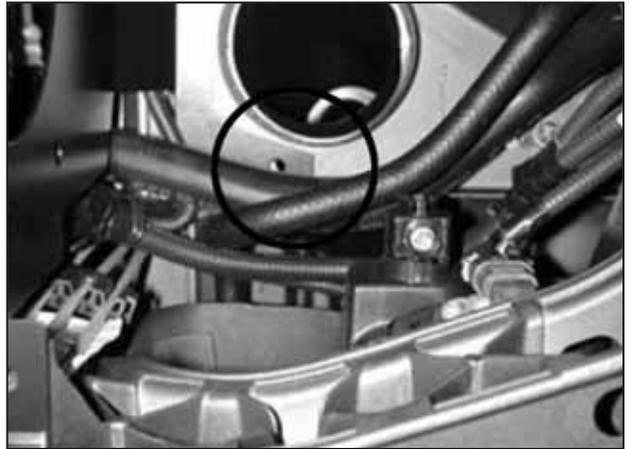
e. Check the clearance around the coolant lines. The mounting tab will pass under the coolant lines. Check for clearance against the wiring harness.
