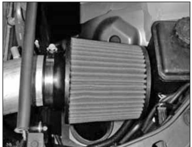
m. Attach the air filter element and tighten the hose clamp.
