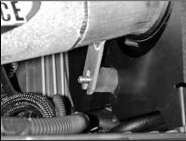
n. Align the bracket with the rubber mount. Once properly positioned, tighten the hose clamp securing the intake pipe to the throttle body.
