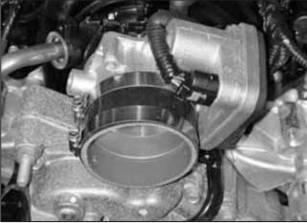
b. Attach the 2" long coupler onto the throttle body with the provided hose clamps. Tighten the throttle body side hose clamp.
