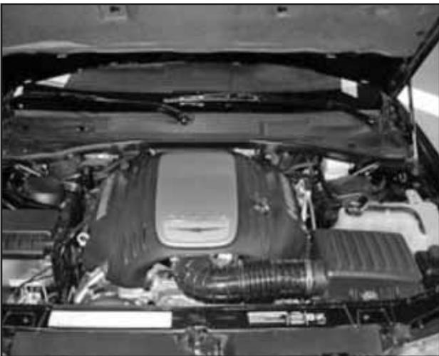
Factory air box system installed
